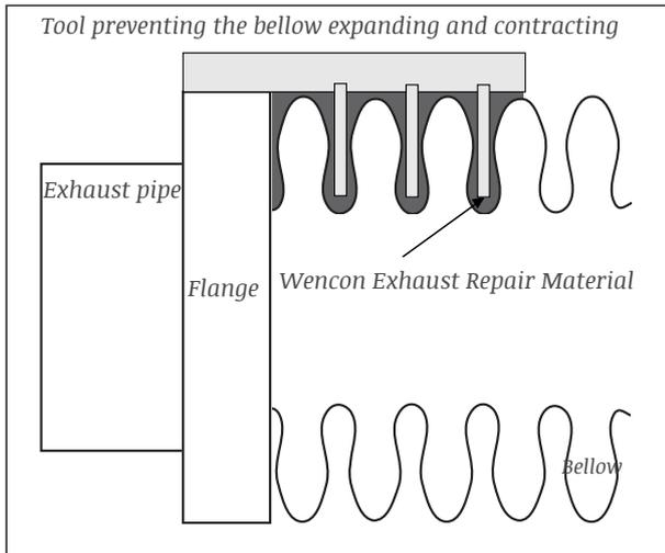
Repair of Bellow can be done as an emergency repair. Below description will guide you through the steps.
