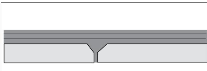
1. Drill a hole in each end of the crack, to prevent the crack elongating.
