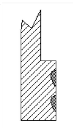
Wencon can provide a solution to repair of wet liners for engines. Corrosion on the outside of the liner, and deterioration of the metal surface of the O-ring seats in either the top or the bottom.
