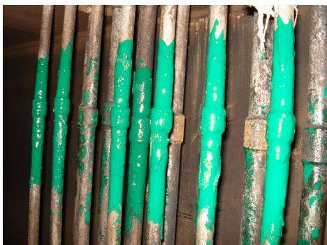
Heating coils often leak in the welding sleeve joints, due to the use of improper welding material. Heavily pitted pipe surfaces are often seen in the bottom area, and they are normally caused by the combination of bad steel – aggressive media- and high surface temperature.
