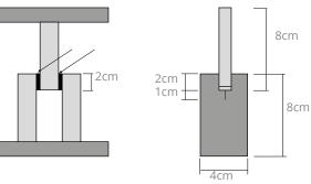
The shear adhesion is determined using the following testing machine: Wolpert, type TT 1220 25 kN. The shear adhesion is calculated according to following formula:
