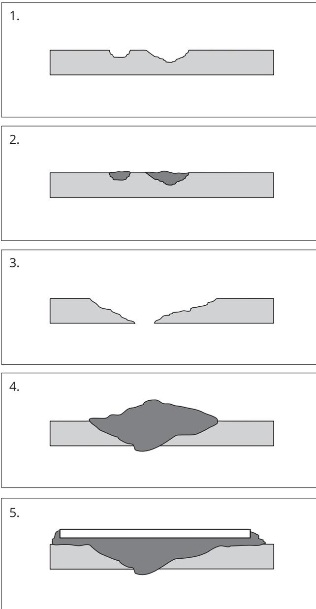
Corrosion attack on deck can be refurbished using Wencon products. Wencon products have a penetration time of more than 15 years, and has an outstanding adhesion to metals.
