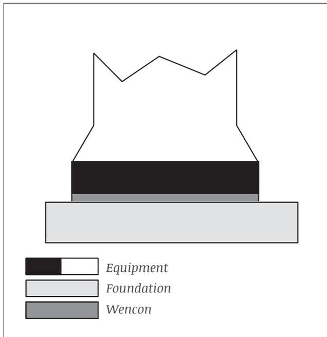
Shocking, casting of resins for the purpose of creating a total fitness between foundation and a piece of equipment, has become more common in the marine industry.
