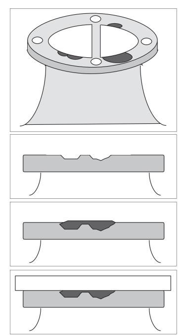
Corroded flanges can be repaired, using Wencon compound. The obvious way would be by shut blasting the flange, applying of Wencon, letting it cure, and machine the flange to size. This method is not always possible, so below find a guide how to do the application on site.
