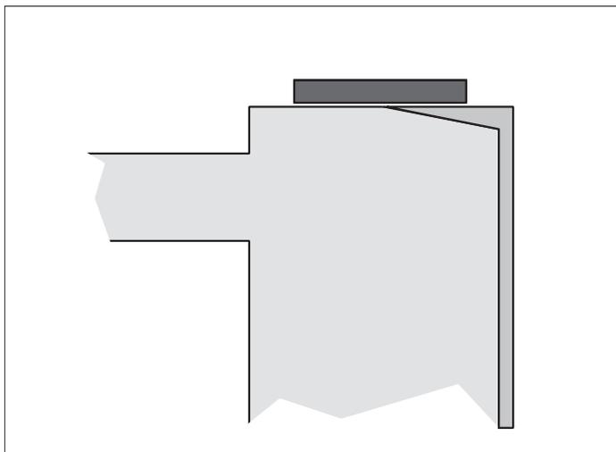
After curing, grind or turn to obtain a smooth packing surface.
