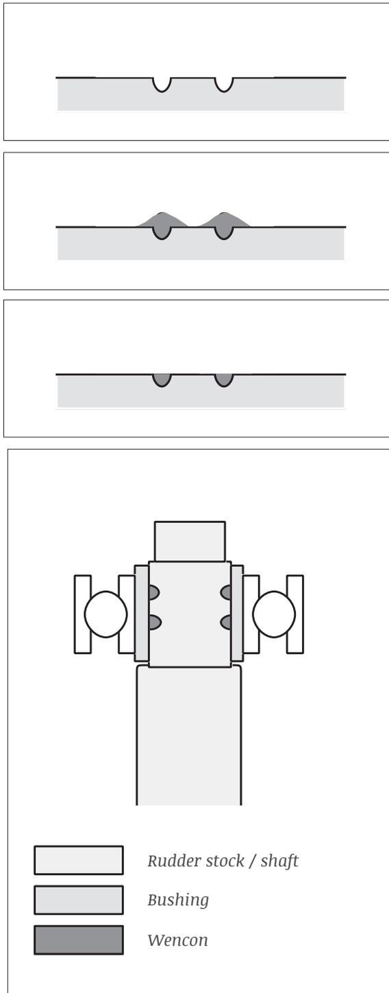
When removing a bushing, from a rudder stock or any other shaft, there might be created scores. In most cases, this damage can be repaired with Wencon.
