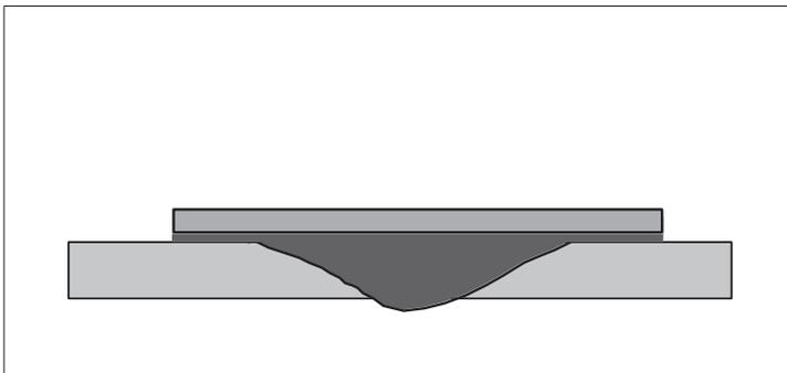
3. For extra security, it is advisable to reinforce the application by the means of a steel plate, grit blasted or ground on one side, and fixed into the Wencon before curing. If the surface of the substrate is shaped, give the plate the approximate same shape before bedding it into the repair. Make sure, that the plate will get in good contact with the Wencon material.
