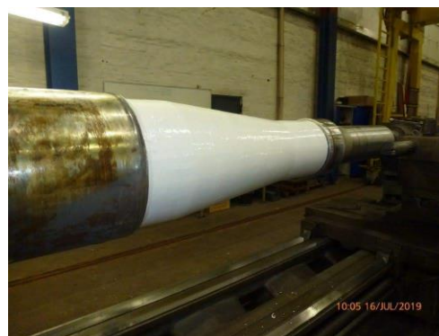
Application of first layer Protective Coatings White completed
