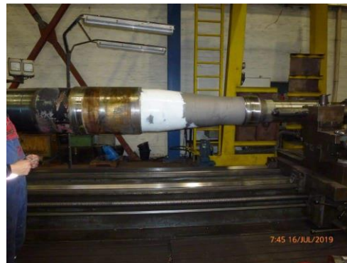
Application of first layer of Wencon Protective Coating White in progress
