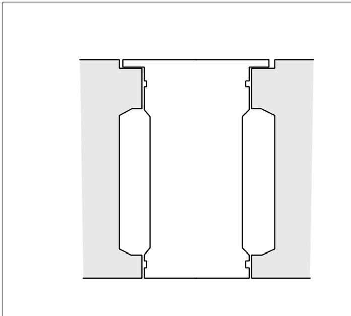
A typical example of a small damage, having a substantial effect is the corroding of the surface that supports an O-ring between the wet liner and the engine block.
