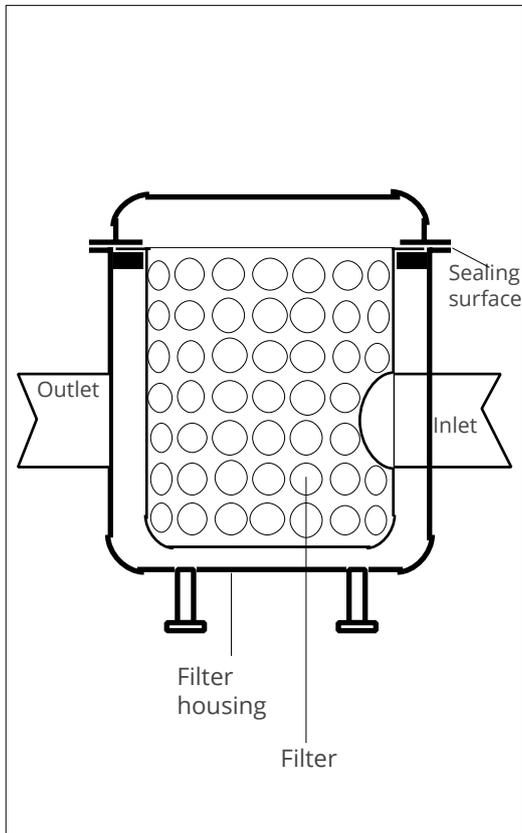
Sea water filters are very varied in appearance, but despite this they contain the same components internally: a filter housing, a filter, an inlet, an outlet, and a sealing surface between filter and housing.
