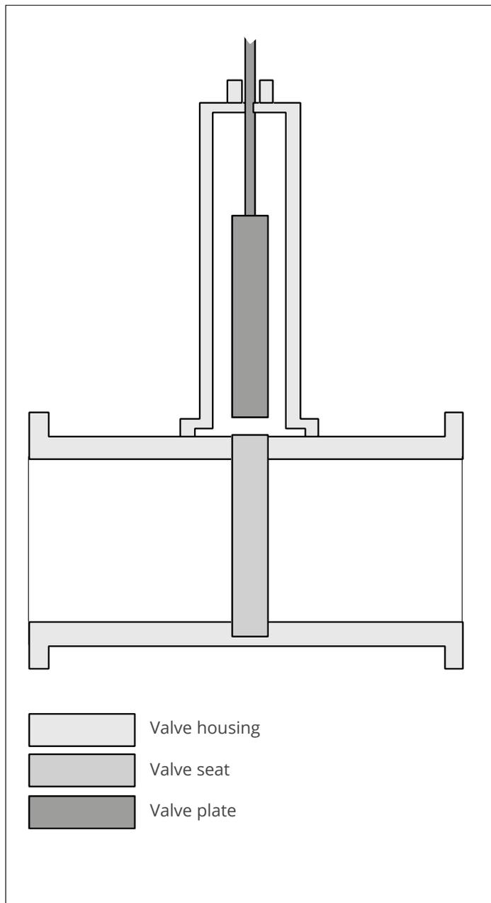
Leaks in valves often occur, due to corrosion in the seating. As a rule the valve is constructed using a number of different metals. Therefore there is every possibility of light acidic agents, such as sea water, causing bimetallic corrosion.
